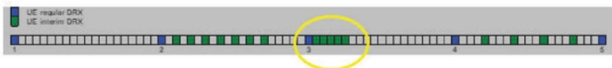
Figure 5: Simplified illustration of regular and interim DRX functionality in time.
